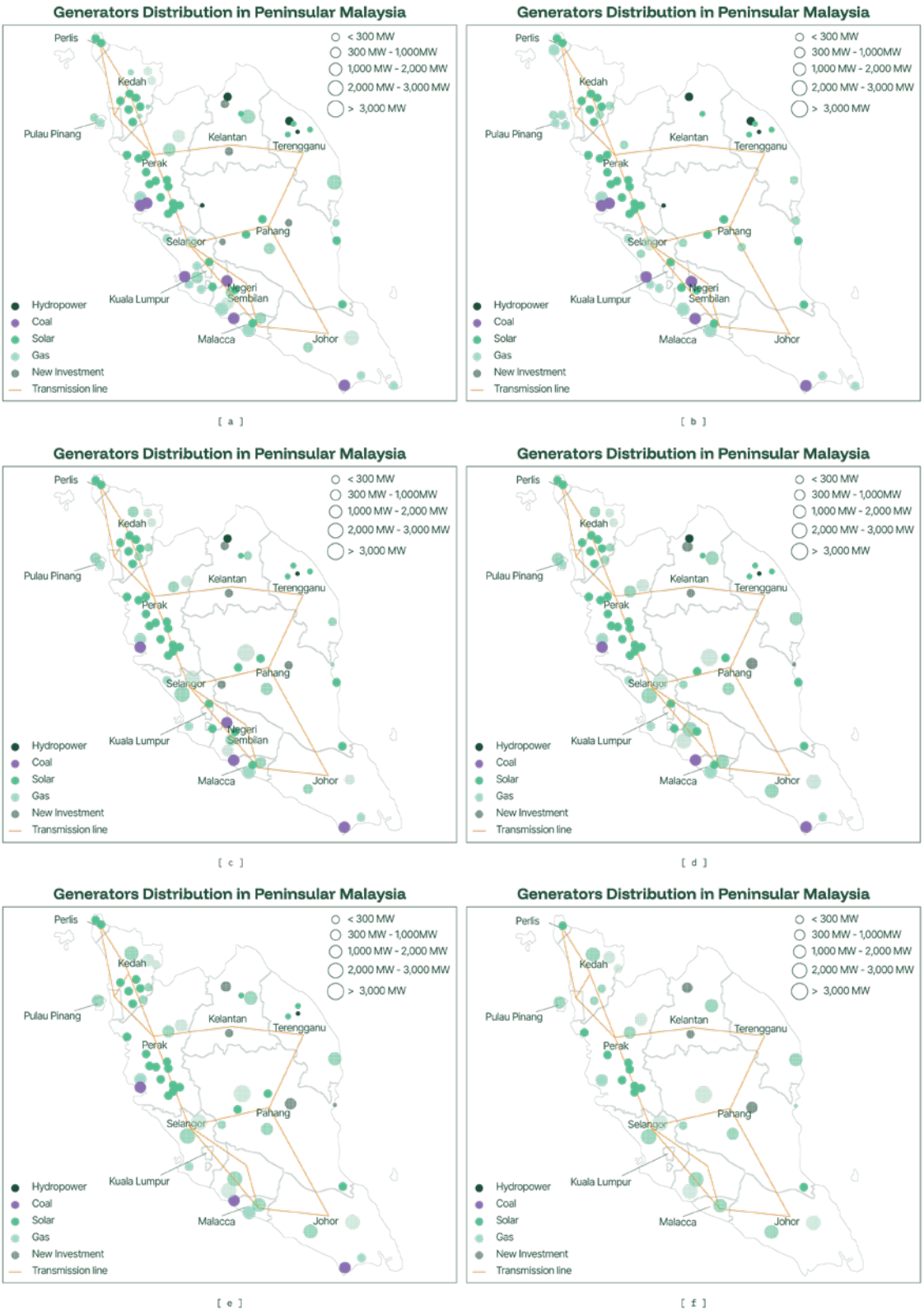
Fig. 4. Distribution of generators in Peninsular Malaysia: (a) 2025, (b) 2026–2030, (c) 2031–2035, (d) 2036–2040, (e) 2041–2045 and (f) 2045–2050
